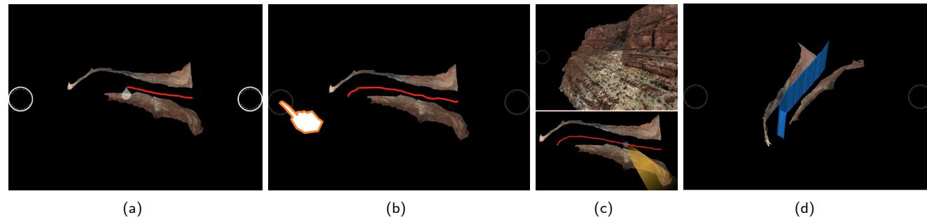
**Figure 1:** The creation of a navigation surface. In (a) the user sketches a path from top view, (b) confirms the selection, and (c) enters navigation mode (bottom shows camera location and point-of-view). In (d) the navigation surface is displayed from an oblique angle.
