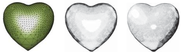
Fig. 9 Heart generated by the implicit function f(x, y, z) = (2x^2 + y^2 + z^2 - 1)^6 - (0.1x^2 + y^2)z^3 . Left from right: triangulated with the method described in [23] and hatched using different spotlight's directions.
