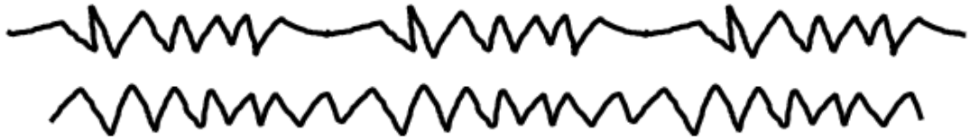
Figure 6.6: Fixing repetition of a style by dropping end points. The smooth areas between the three repetitions of the style (top) are eliminated by dropping start and end points of the extracted style. The result is a seamless repetition (bottom).
