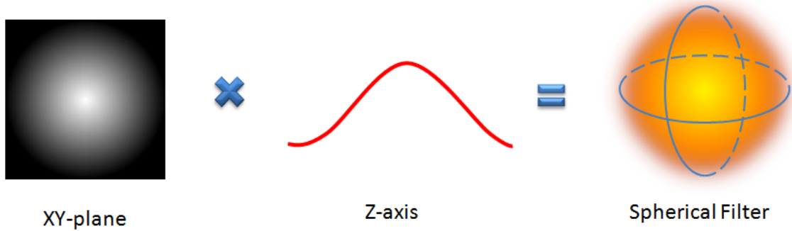
Figure 3.7: Combining 2D Gaussian function in the XY -plane and 1D Gaussian function in the Z -axis to form a spherical filter that reconstructs a 3D Gaussian function.
