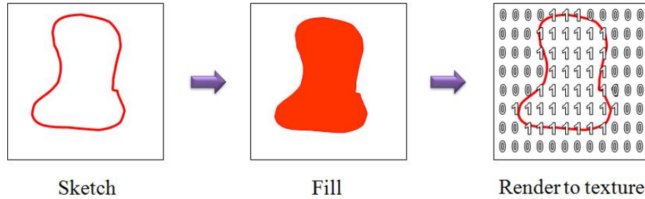
Figure 3.9: Generating the computational mask using the stencil buffer.
