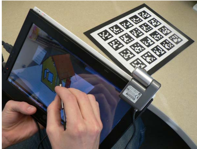
Figure 5.5: Mixed reality using the lens metaphor with sketchpad and napkin
