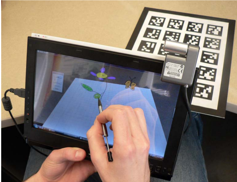
Figure 1.2: Napkin Sketch : creating a 3D sketch using sketchpad and napkin
