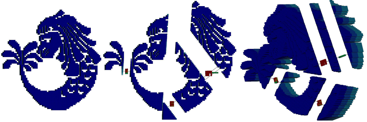
Figure 6.1: Exploded view diagrams applied to 3D grid (from left to right): the whole grid; the final result with primary objects exposed; another final result from a different view angle.
