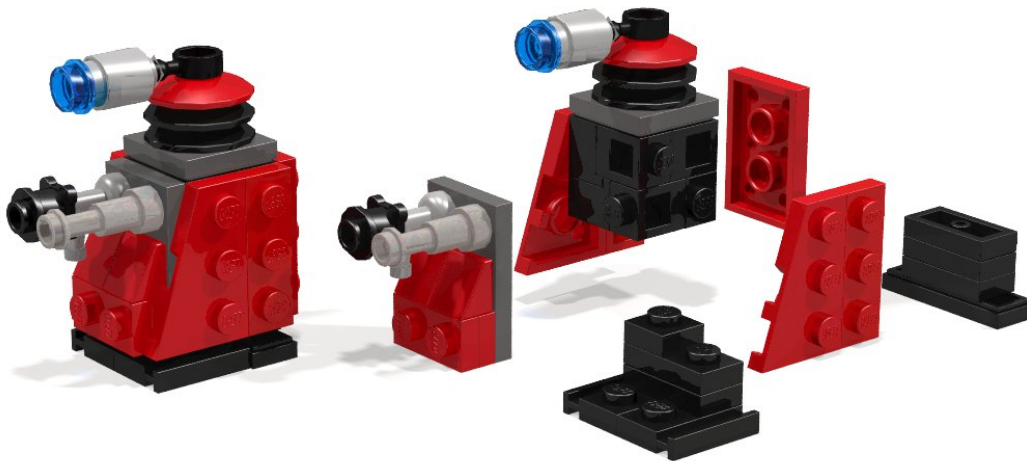
Figure 1.5: Exploded View: (left) the whole object; (right) object of interest is exposed by splitting the object.
